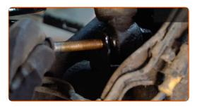
Screw in the lower fastener of the shock absorber. Use a drive socket #E14.
