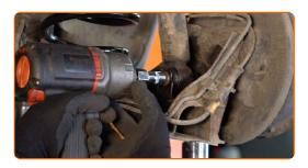
Remove the fastening bolt.
