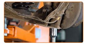
Unscrew the lower fastener of the shock absorber. Use a drive socket #E14.
