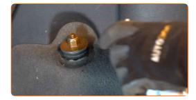
Install the protective cap of the shock absorber mount.
