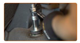
Treat the shock absorber fasteners. Use copper grease.
