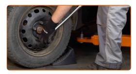
Tighten the top shock absorber fastening. Use a drive socket #16. Use a shock absorber socket DDNº6. Use a torque wrench. Tighten it to 65 Nm torque.
