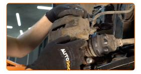
Tighten the brake caliper fasteners. Use a drive socket #12. Use a torque wrench. Tighten it to 27 Nm torque.
