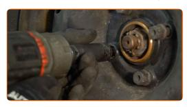
Lower the car and working in a cross order, tighten the wheel bolts. Use a torque wrench. Tighten it to 110 nm torque.
