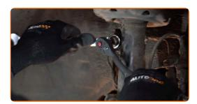
Unscrew the fastener connecting the stabilizer link to the shock strut. Use a combination spanner #18. Use a drive socket #8. Use a ratchet wrench.
