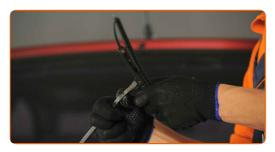
Remove the blade from the wiper arm.
