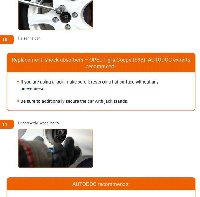
Loosen the wheel mounting bolts. Use wheel impact socket #17.
