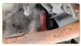
Detach the oxygen sensor connector.
