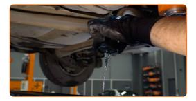
Remove the retainers of the fasteners of the fuel filter tubes.
