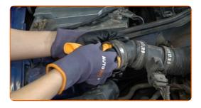
6 Release the air filter cover clips.
