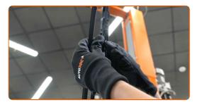
Remove the blade from the wiper arm.
