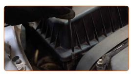
Unplug the mass air flow sensor connector.
