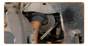
9 Place the V-ribbed belt on the tensioner pulley.
