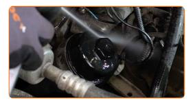
Unscrew the filter housing cap together with the old filter element. Use a drive socket #32. Use a ratchet wrench.
