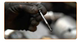
Tighten the fasteners of the fuel filter cover. Use Torx T30. Use a ratchet wrench.
