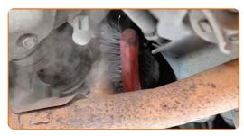
Detach the oxygen sensor connector.
