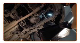
Unscrew the fasteners of the transmission fluid pan. Use a drive socket #11. Use a ratchet wrench.
