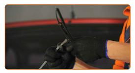
Remove the blade from the wiper arm.
