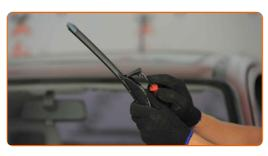
Remove the blade from the wiper arm.
