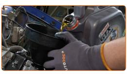
Replacement: engine oil and filter – OPEL REKORD E (17\_-19\_, 11\_, 14\_, 16\_).
