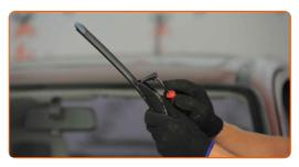
Remove the blade from the wiper arm.
