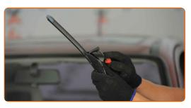
Remove the blade from the wiper arm.
