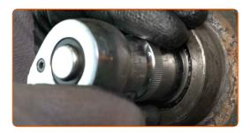
Remove the wheel bearing washer. Use a crowbar.
