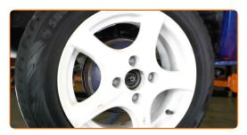
Adjust the axial clearance by tightening the adjusting nut. Use a drive socket #24. Use a torque wrench. Tighten it to 20-25 Nm torque.
