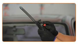
Remove the blade from the wiper arm.
