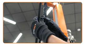
Remove the blade from the wiper arm.
