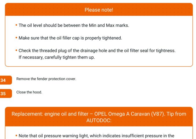
lubrication system, may be on for a longer time than usual. After a few seconds, the oil will fill all the channels, and the light will go out.
