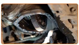
Replacement: manual gearbox oil – OPEL Omega A Caravan (V87). Tip from AUTODOC:
