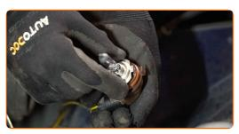
Replacement: headlight bulb – OPEL Movano B Platform / Chassis (X62).
