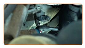
6 Remove the fastening bolt.
