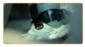
Tighten the fastener of the camshaft position sensor. Use a 10 mm socket. Use a torque wrench. Tightening torque: 10 N·m.
