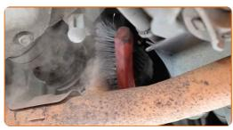
Detach the oxygen sensor connector.
