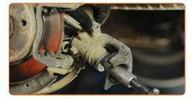
17 Install the brake caliper and fix it.
