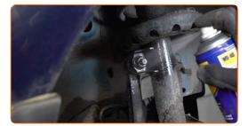
Unscrew the nut and remove the stabilizer rod from the shock strut. Use a combination spanner #19. Use a drive socket #18.
