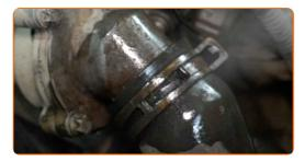
Loosen the clamps of the coolant hoses. Use clic-R collar pliers.
