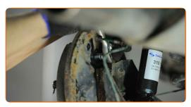
Remove the brake cylinder from the backplate. Use a crowbar.
