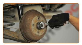
9 Remove the brake drum.
