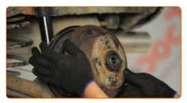
Screw in the wheel hub fastener. Use a combination spanner #24. Use a ratchet wrench.
