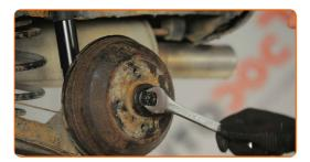
Install the cotter pin of the hub bearing fastening nut. Use round-nose pliers.
