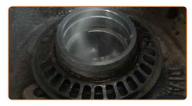
Install a new wheel bearing outer race in the brake drum. Bush and bearing driver set.
