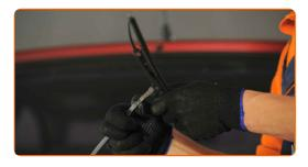
Remove the blade from the wiper arm.
