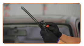
Remove the blade from the wiper arm.
