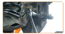
Remove the caliper bracket.
