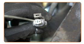
Attach the ABS sensor connector.
