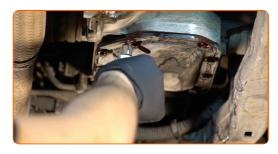
10 Remove the transmission fluid pan.
