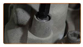
Remove the brake caliper.
