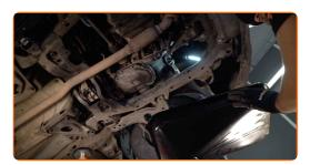
Unscrew the fasteners of the transmission fluid pan. Use a drive socket #11. Use a ratchet wrench.
