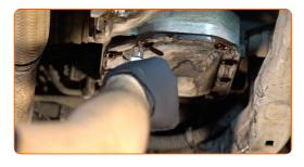
10 Remove the transmission fluid pan.
