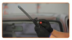
Remove the blade from the wiper arm.
