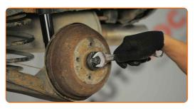
9 Remove the brake drum.
