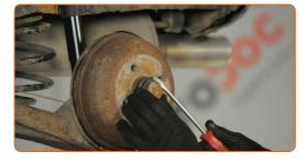
Remove the cotter pin securing the hub nut. Use round-nose pliers.
