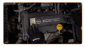
Detach the connector from the ignition coil. Use a flat screwdriver.
