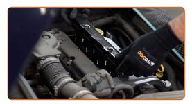
Tighten the ignition coil fastening. Use Torx T30. Use a torque wrench. Tighten it to 15 nm torque.
