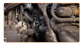
Insert the funnel. Pour new transmission fluid in the gearbox through the breather hole. Required amount of oil: 1.6 L.
