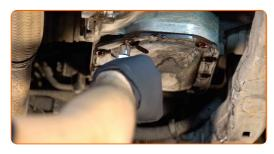
10 Remove the transmission fluid pan.
