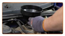
Pour coolant in the coolant reservoir.
