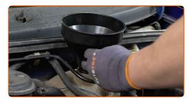
Pour coolant in the coolant reservoir.
