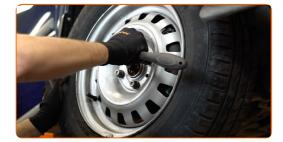
Lower the car and working in a cross order, tighten the wheel bolts. Use a torque wrench. Tighten it to 110 Nm torque.
