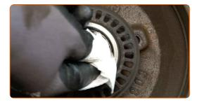
Remove the inner race of the wheel bearing from the brake drum. Use a universal puller.
