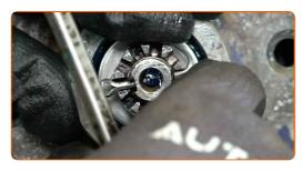
Install the cap of the hub nut. Use a rubber mallet.
