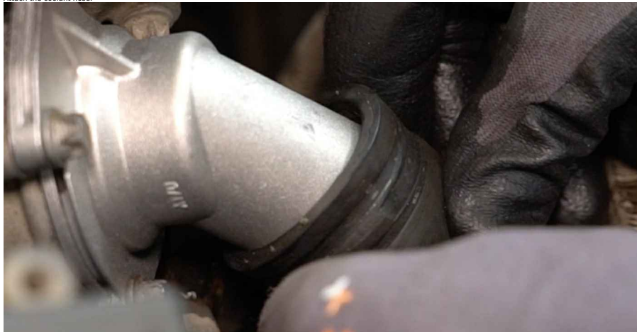
28 Attach the coolant hose.
