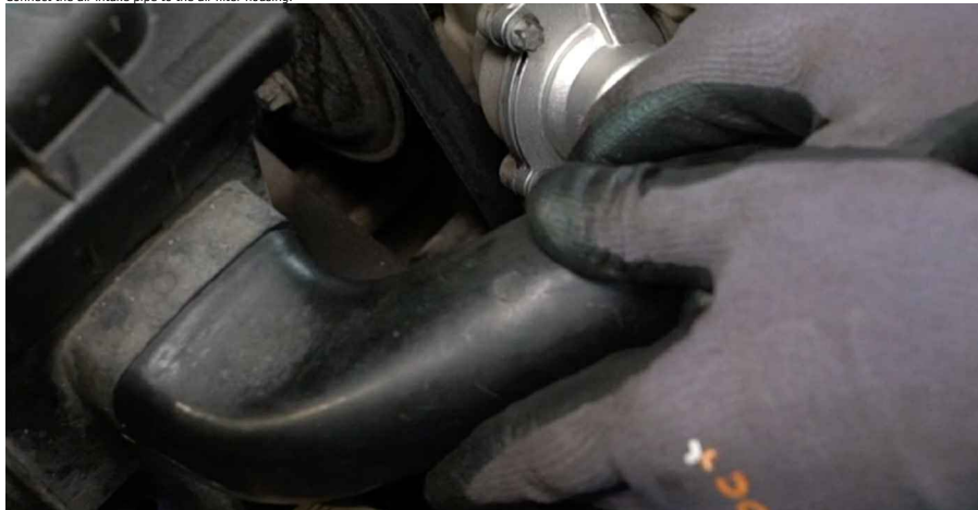
32 Attach the clip on the air filter intake hose.
