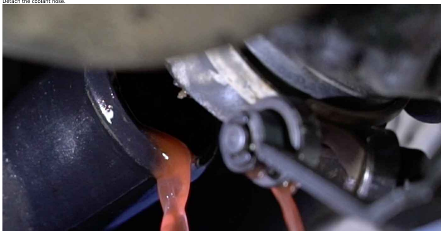
8 Detach the coolant hose.
